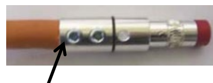
Cable and sleeves mounted on a contact
